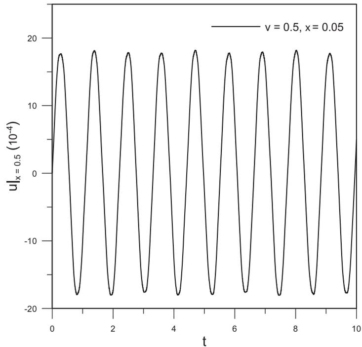
Fig. 7. Dimensionless transverse displacement  $u(x,t)$  of a clamped axially moving beam at  $x=0.5$  for  $\nu=0.5$  and  $\xi=0.05$ .
