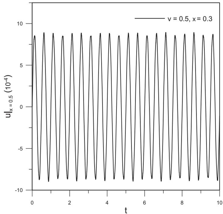
Fig. 8. Dimensionless transverse displacement  $u(x,t)$  of a clamped axially moving beam at  $x=0.5$  for  $\nu=0.5$  and  $\xi=0.3$ .
