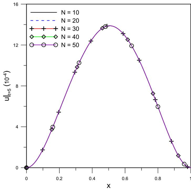
**Fig. 1.** GITT solutions with different truncation orders  $N$  for the dimensionless transverse displacement  $u(x,t)$  of a clamped axially moving beam at  $t = 5$  for  $\nu = 0.15$  and  $\zeta = 0.1$ .
