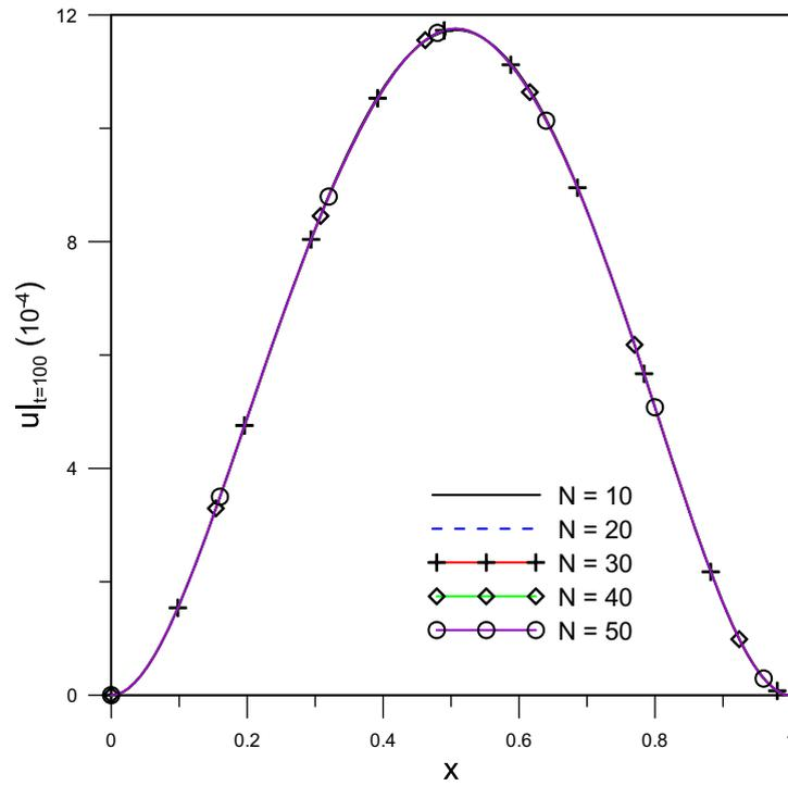
Fig. 3. GITT solutions with different truncation orders  $N$  for the dimensionless transverse displacement  $u(x,t)$  of a clamped axially moving beam at  $t = 100$  for  $\nu = 0.15$  and  $\zeta = 0.1$ .
