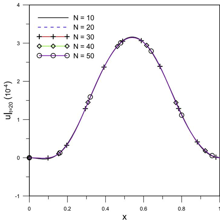
**Fig. 2.** GITT solutions with different truncation orders  $N$  for the dimensionless transverse displacement  $u(x,t)$  of a clamped axially moving beam at  $t = 20$  for  $\nu = 0.15$  and  $\zeta = 0.1$ .
