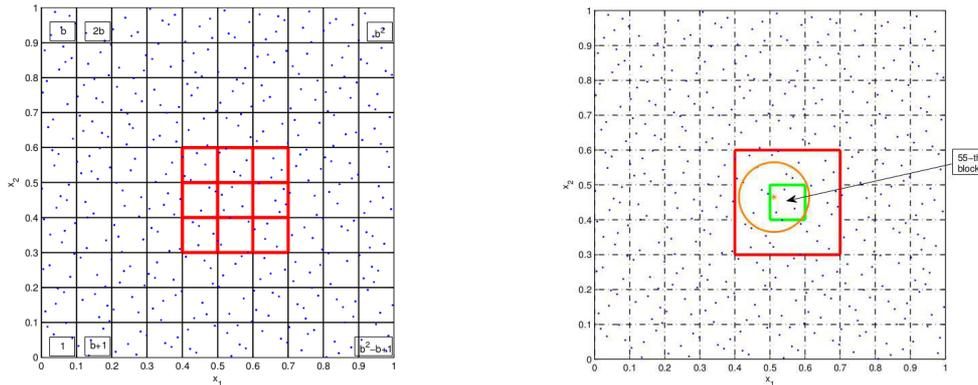
Figure 2: Example of block-based structure applied to interior collocation points (blue): to left the partitioning structure with the  $k$ -th block and its eight neighboring blocks (red); to right the  $k$ -th block (green, with  $k = 55$ ) and a neighborhood associated with a point denoted by  $\star$  (orange) belonging to the  $k$ -th block.
