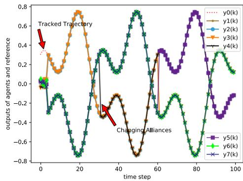
Figure 15. Tracking performance of MASs with switching topologies and  $\theta=0.2$  at 370th (example 3).
