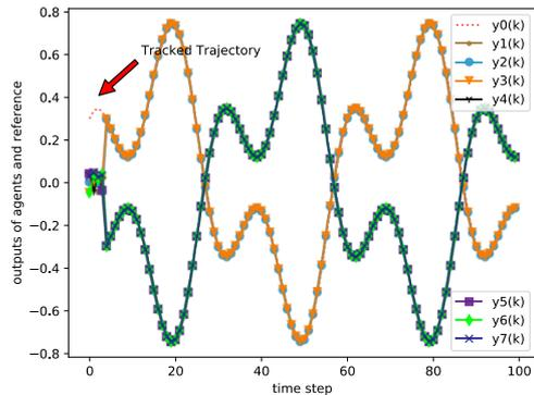
Figure 13. Tracking performance of MASs with fixed topology and  $\theta=0.2$  at 370th (example 3).
