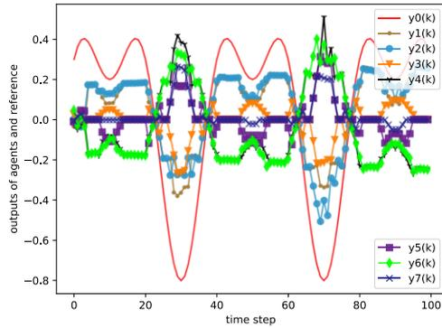
Figure 6. Tracking performance of MASs with  $\theta=0.2$  at 10th (example 1).
