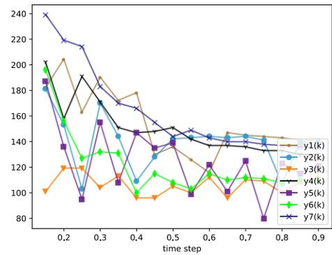
Figure 9. Convergence speed of MASs with different  $\theta$  (example 1).
