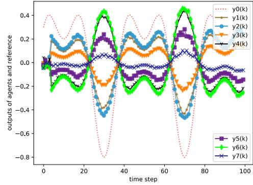
Figure 3. Tracking performance of MASs with  $\theta=0.9$  at 10th (example 1).
