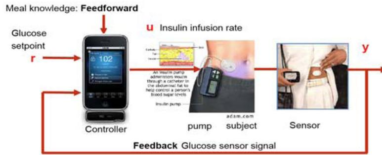
**Fig. 1.** Block diagram of a closed-loop artificial pancreas (adapted from Bequette, 2005). The use of meal feedforward control is often called “meal announcement.”
