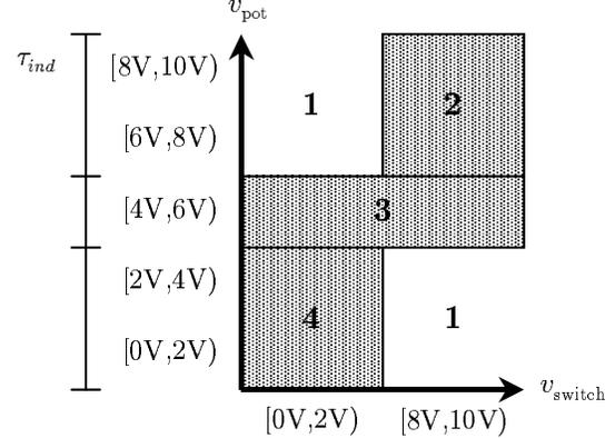
Figure 2: Partition  $\Sigma(R, \tau_{obs}, \tau_{target})$  for the pedal position sensor example. The partition consists of four elements numbered 1, 2, ..., 4. Applying theorem 1 yields the distinctions for  $v_{pot}$  shown on the left-hand side of the figure.
