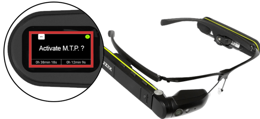
Figure 3: The Vuzix m300 smart glasses used for the TraumaTracker prototype. In the circle, an example of a warning on received by the Trauma Leader: the border color categorize the warning level and the message in the middle define the content of it. In this case, the warning to request to activate the M.T.P. according to the rule 2.
