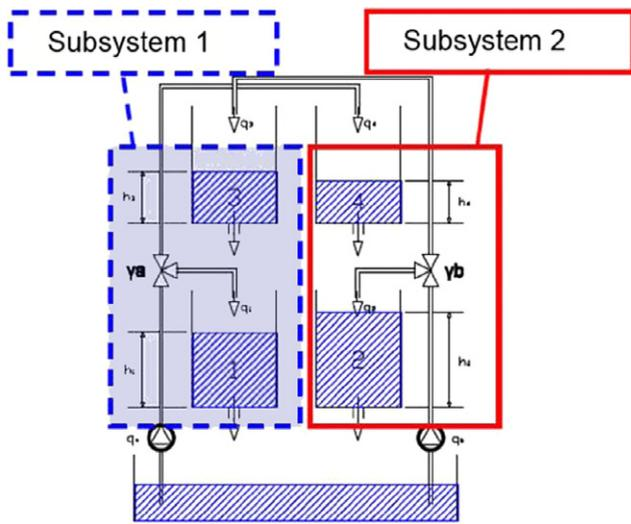
Fig. 3. The four-tank process: two distributed subsystems.
