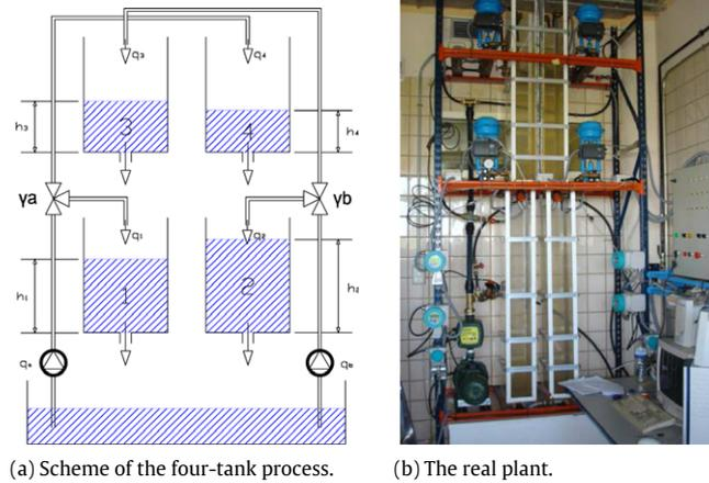
Fig. 2. The four-tank process.
