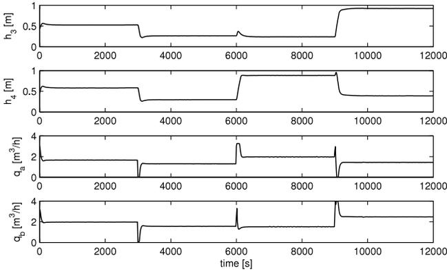
Fig. 6. Time evolution of  $h_3$  and  $h_4$  and of the control inputs  $q_a$  and  $q_b$ .
