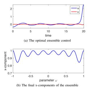
Fig. 4. (a) The optimal ensemble control that steers an ensemble of Bloch systems with  $\omega \in [-1,1]$  from  $X_0(\omega) = (0,0,1)^T$  to a neighborhood of  $X_d(\omega) = (1,0,0)^T$ . The weighted matrix  $R = I_3$ . (b) The final states  $X(20, \omega)$  for 81 spin systems (blue) with their frequencies uniformly spaced within [-1,1] following the control displayed in (a).
