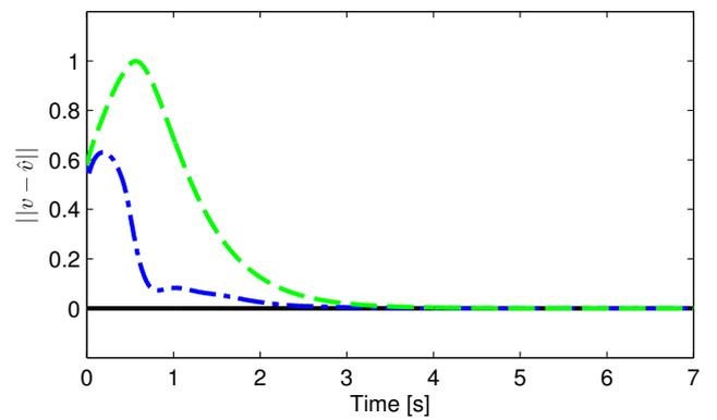
Fig. 6. Observer estimation error norm  $\|v - \hat{v}\|$  when using the controllers of Theorems 7 (dashed-dotted blue) and 8 (dashed green).
