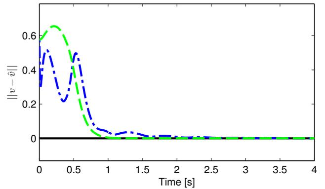
Fig. 7. Observer estimation error norm  $\|v - \hat{v}\|$  when using the controllers of Theorems 7 (dashed-dotted blue) and 8 (dashed green) with faster convergence times.
