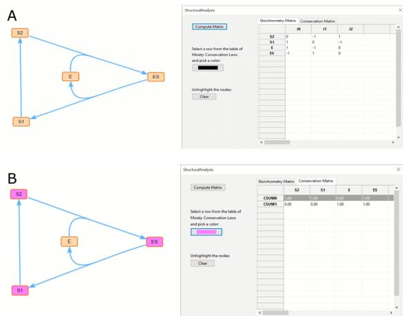
**Figure 4: Structural analysis plugin.** A. Compute and show the stoichiometry matrix. B. Compute the conservation matrix and highlight the nodes of a conserved moiety.
