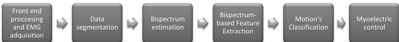
Fig. 1. Block diagram of the overall myoelectric control system.
