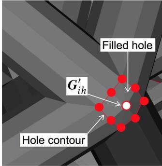
Figure 15: Hole filling using barycenter projection for  $Val_i = 4$ .
