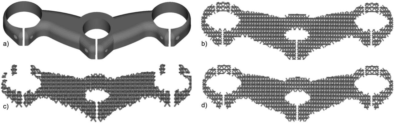
Figure 17: Triangulation of a lattice structure inserted in an industrial T-fork: (a) triangle mesh used to generate the lattice cells of size  $7 \times 7 \times 7$ , (b) MCM triangulation: 1130400 triangles, (c) CDT triangulation: 229888 triangles, (d) LSLT triangulation: 126488 triangles.
