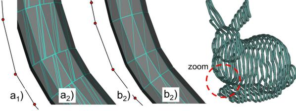
Figure 10: Comparison between: (a1) the lattice structure made of nodes and beams and (a2) its associated classic boolean result (non manifold and addition of triangles), (b1) the lattice structure and (b2) our associated special boolean operator result (manifold and no added triangles) for  $Val_i = 2$  on the Stanford bunny lattice mesh.
