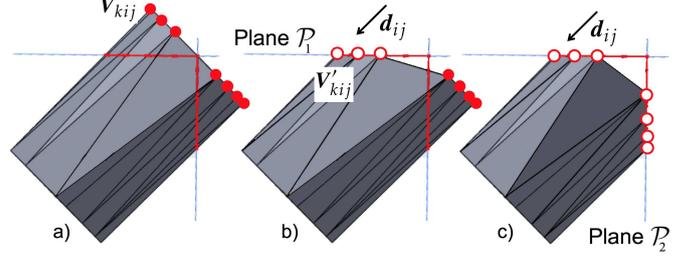
Figure 12: Different steps of our boolean operator : (a) initial section with intersection planes, (b) first displacements of vertices toward the first plane (gap creation), (c) second displacements toward the second plane with hole appearance.
