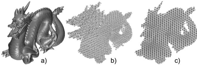
Figure 18: Triangulation of a lattice structure inserted in the Stanford dragon: (a) initial triangle mesh used to generate the lattice cells of size  $2 \times 2 \times 2$ , (b) MCM triangulation: 7462036 triangles, (c) LSLT triangulation: 315728 triangles.
