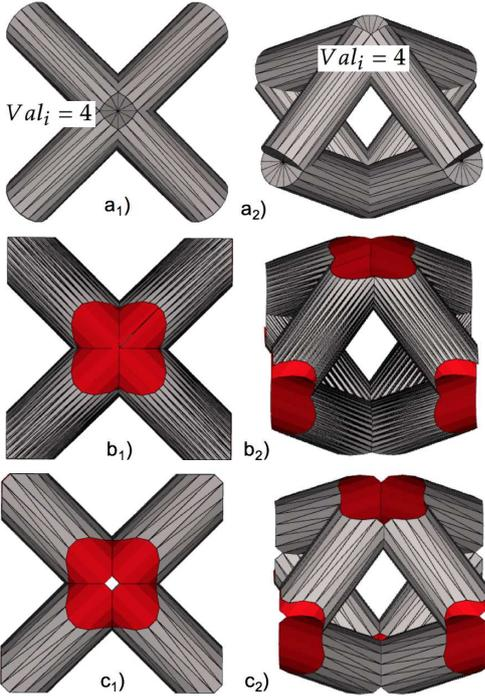
Figure 11: Top and isometric views for  $Val_i = 4$  on a lattice cell mesh. Results comparison between : (a1) and (a2) initial cylinders with a given precision, (b1) and (b2) classic boolean result (non manifold and added triangles), and (c1) and (c2) our special boolean operator result (manifold and no added triangles)
