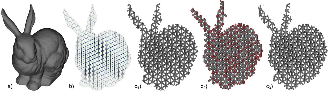
Figure 16: Triangulation of a lattice structure inserted in the Stanford bunny: (a) initial triangle mesh to be filled in by a lattice structure, (b) lattice cells of size  $7 \times 7 \times 7$ , (c<sub>1</sub>) MCM triangulation: 924644 triangles, (c<sub>2</sub>) CDT triangulation: 377106 triangles, (c<sub>3</sub>) LSLT triangulation: 94872 triangles.
