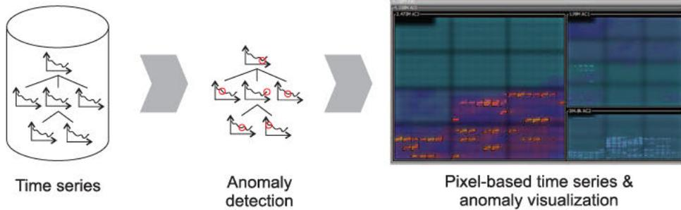
Fig. 1. The input set of hierarchical time series is processed by anomaly detection methods. The resulting anomaly values are visualized together with the time series values by pixel-based techniques. The visualization combines the raw time series with boosting techniques like highlighting and blurring for the anomaly scores.
