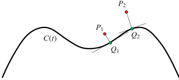
Figure 5: Illustration of Example 1:  $Q_1$  and  $Q_2$  are the exact projective points of  $P_1 = (381, 252)$  and  $P_2 = (332, 200)$ . The control points and knot vector of  $C(t)$  are  $\{(100, 100), (140, 196), (200, 240), (260, 164), (340, 164), (400, 240), (460, 196), (500, 100)\}$  and  $(0, 0, 0, 0, 0.2, 0.4, 0.6, 0.8, 1, 1, 1, 1)$ , respectively.
