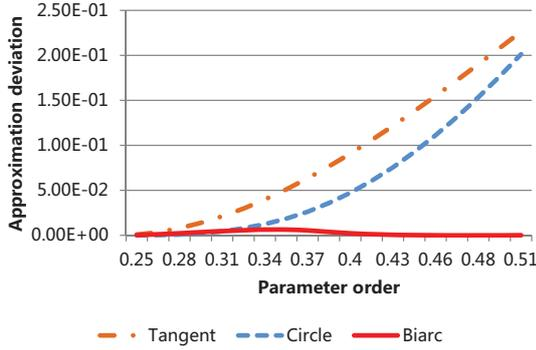
Figure 2: Approximation deviation comparison in Figure 1. Abscissa is the parameter of the moving point on the original curve. Ordinate is the distance from the moving point to approximation curve.
