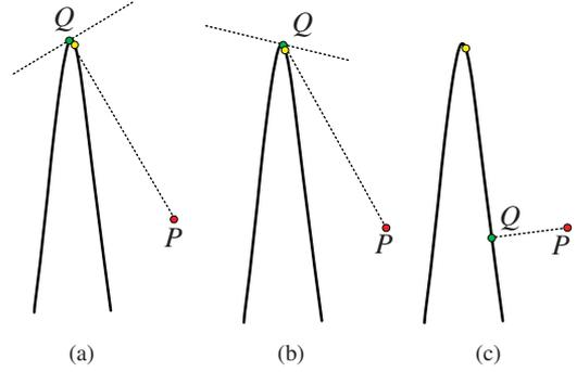
Figure 6: Illustration of Example 2. The yellow point is the initial projection. The control points of the Bézier curve are  $\{(0, 0), (110, 1000), (90, 1000), (200, 0)\}$ : (a) projection result  $Q$  of NRA and its tangent; (b) projection result  $Q$  of SOA and its tangent; (c) projection result  $Q$  of SOIBA.
