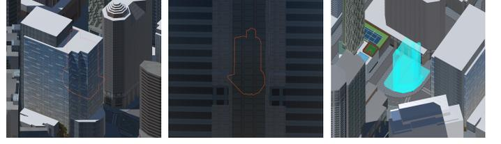
**Fig. 6.** Effects of different energy terms on viewport optimization. **Left:** camera target distance ( $E_1$ ) and camera obstruction ( $E_2$ ) only cause occlusion of the target building. **Middle:** camera target distance ( $E_1$ ) and view occlusion ( $E_3$ ) only block the camera. **Right:**  $E_1 + E_2 + E_3$  produces optimal viewport for the target building.
