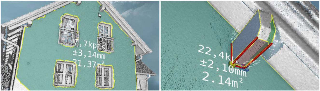
**Figure 8:** Zoom out (left) to obtain a planar regression of the entire house wall. Zoom in (right) to capture details in a local part of the wall.
