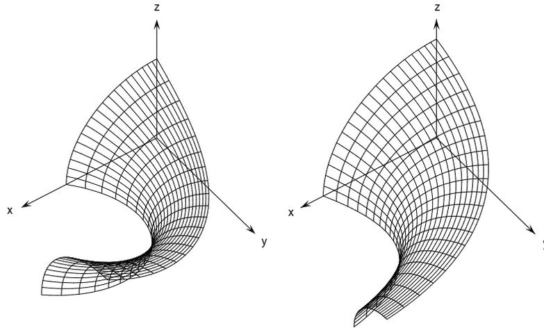
Figure 7: Generalized conical swept surfaces generated by a circular profile curve  $\mathbf{p}(u)$  in the  $(x, z)$  plane and a PH quintic sweep curve  $\mathbf{s}(v)$  in the  $(x, y)$  plane, using the quadratic scaling function (33) with coefficients  $(c_0, c_1, c_2) = (1.0, 0.0, 1.0)$  on the left, and  $(c_0, c_1, c_2) = (1.25, 0.75, 0.50)$  on the right.
