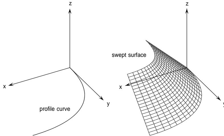
Figure 3: The offset–translation swept surface (20) generated by a PH quintic profile curve  $\mathbf{p}(u)$  in the  $(x, y)$  plane and offset distance function  $d(v) = v$ .
