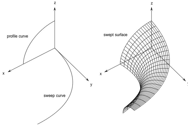
Figure 6: The generalized conical swept surface (30) generated by a circular profile curve  $\mathbf{p}(u)$  in the  $(x, z)$  plane and a PH quintic sweep curve  $\mathbf{s}(v)$  in the  $(x, y)$  plane, with factors  $c_0 = 1$  and  $c_1 = \frac{1}{2}$  in the scaling function (29).
