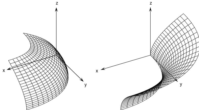
Figure 4: The offset–translation surface generated by the same PH quintic as in Figure 3, using distance functions  $d(v) = v^2$  (left) and  $d(v) = -v^2$  (right).
