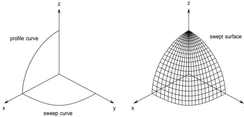
Figure 1: The scaled-rotation surface defined by a circular arc in the  $(x, z)$  plane as the profile curve, and a cubic in the  $(x, y)$  plane as the sweep curve.
