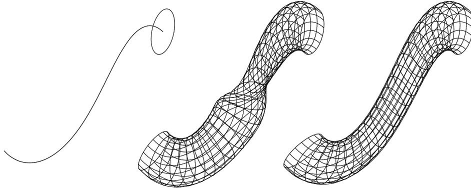
Figure 8: The tubular surface generated by sweeping an ellipse profile curve along an RRMF quintic sweep curve (left). The profile curve lies in the sweep curve normal plane at each point, and within this plane it is oriented using either the Frenet frame (center) or the rotation–minimizing frame (right).
