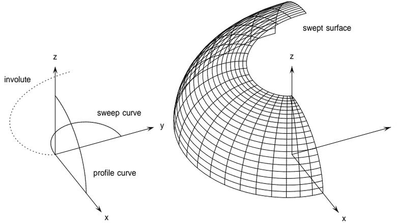
Figure 5: Left: a circle arc in the  $(x, z)$  as the profile curve, and a PH quintic sweep curve in the  $(x, y)$  plane, together with its involute (the dotted curve). Right: the oriented–involute swept surface generated by these two curves.
