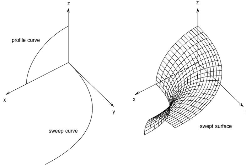
Figure 2: The oriented–translation surface generated by a circular arc profile curve in the  $(x, z)$  plane, and a PH quintic sweep curve in the  $(x, y)$  plane.
