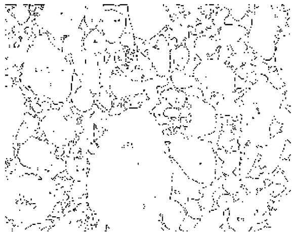
Fig. 5. Perimeter pixels related to thin section shown in Fig. 2. Each black pixel corresponds to perimeter between grey and white areas resulting from original image.
