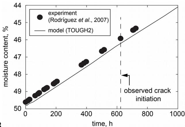
403 404 Fig. 8. Evolution of gravimetric moisture content of sample with thickness of 16mm.
