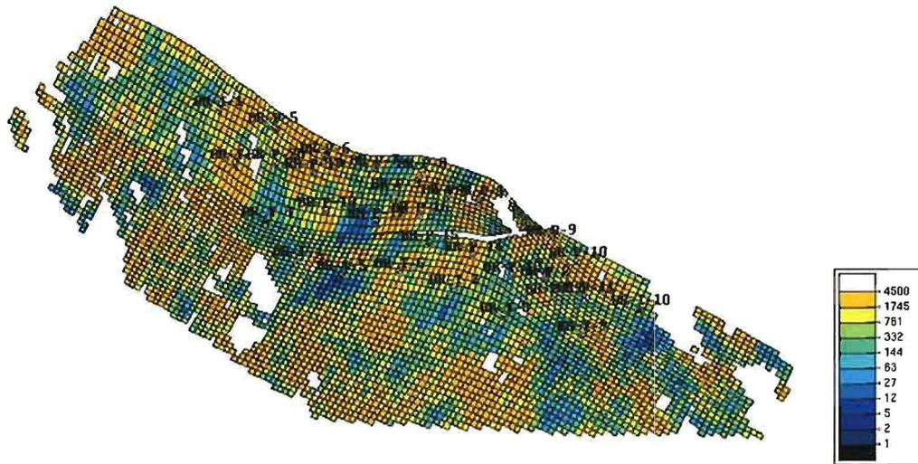
Figure 7: Permeability and well positions on the Brugge reservoir
