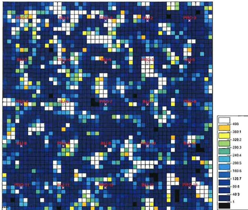
Figure 5: Permeability map of the synthetic oil field
