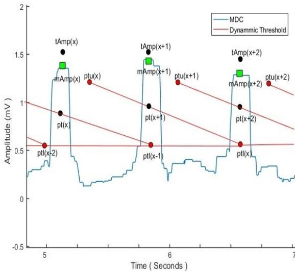
Fig. 6 - Time varying dynamic threshold selection with respect to the MDC
