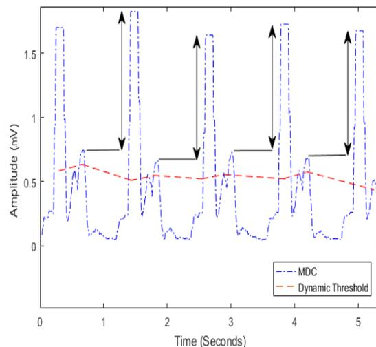
Fig. 10 - Unusually low thresholds on the MDC
