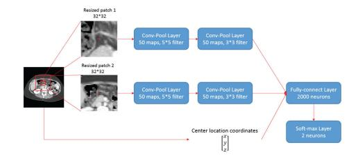
**Figure 4.** Architecture of Segmentation-CNN
