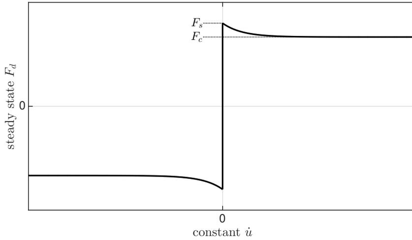
Figure 12: Steady state of the dry friction force versus constant velocity.
