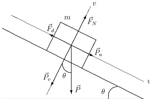
Figure 9: Cube on an inclined plane.
