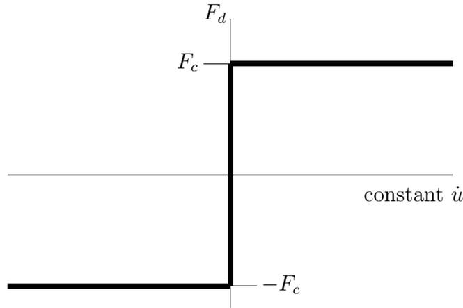
Figure 10: The Coulomb model for dry friction.
