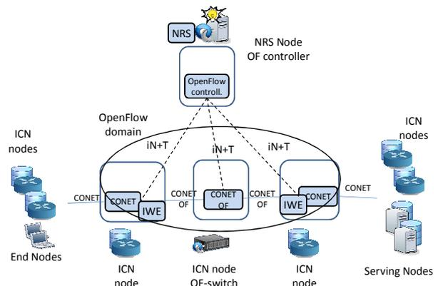
**Figure 5- Reference Interfaces for intra-domain specific SDN functionalities**
