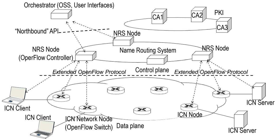
**Figure 3- Information Centric Network based on extended OpenFlow**
