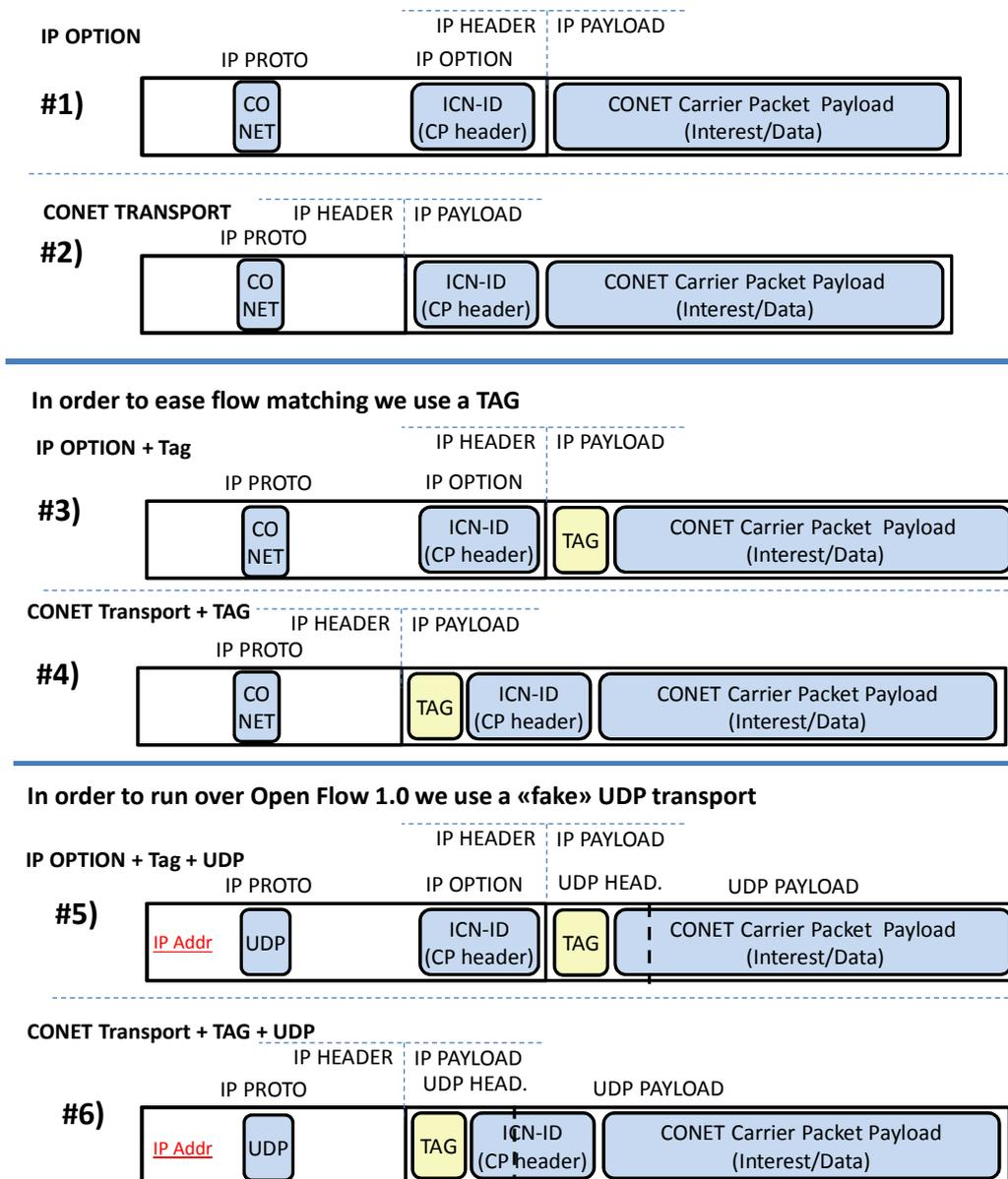
Figure 6- Different choices for CONET packet format
