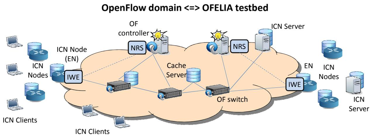
**Figure 7- Details of the OpenFlow 1.0 solution to support ICN**
