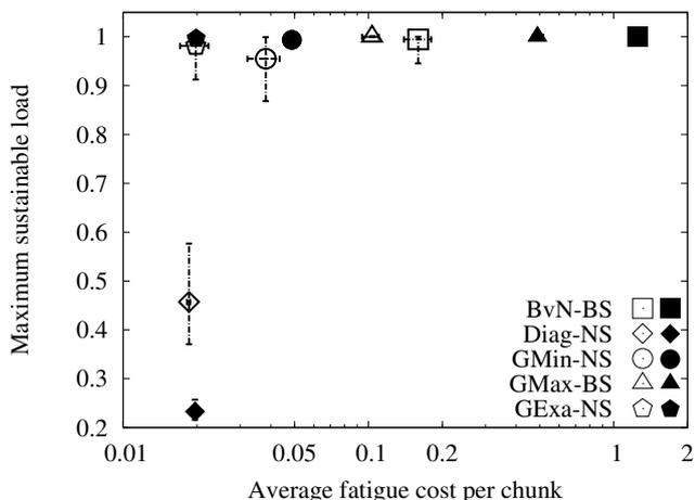
Figure 6: Throughput and fatigue tradeoff under UniAS traffic for  $N = 16$  (white shapes) and  $N = 128$  (black shapes).
