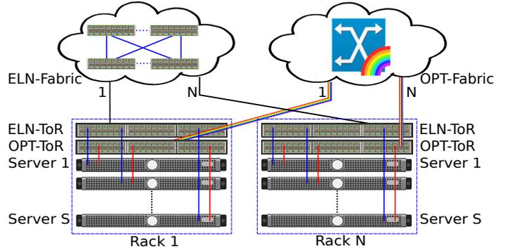
Figure 1: Hybrid data center architecture based on  $N$  ToR racks, each of them hosting  $S$  servers. Each server is connected to both an ELN-ToR switch and an OPT-ToR switch. The former switch accesses an electronic packet switch network (ELN-fabric) and the latter accesses an optical circuit switch network (OPT-fabric). Each fabric has  $N$  bidirectional ports, one for each rack.
