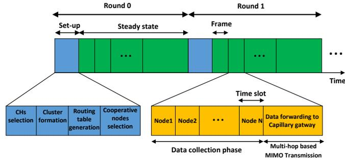
Figure 4: Transmission structure in cluster-based IoT system
