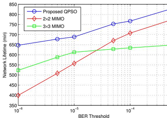
Figure 8: Network lifetime vs. BER threshold
