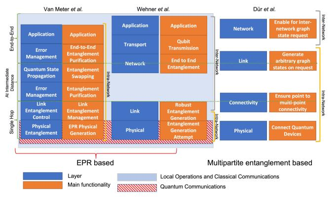
Figure 13: Joint representation of the main contributions toward the Quantum Internet protocol stack: Van Meter et al.'s model (left), Wehner et al.'s model (center) and Dür et al.'s model (right).
