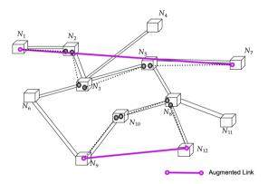
(c) Augmented Graph obtained through entanglement swapping. In the example, nodes  $N_1$  and  $N_7$  are directly connected by an augmented virtual link, although they are not connected in the physical graph nor in the virtual graph.
