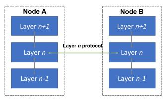
**Figure 2:** Example of a generic layered model for a communication network. Node A and Node B represent two network entities implementing more than one layer. Layer n of Node A offers its functionalities to layer n+1 and uses the functionalities of layer n-1. Additionally, Node A's layer n can directly interact with Node B's layer n through a specific protocol.
