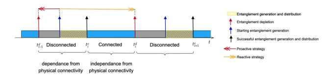
Figure 7: Visual representation of the dynamics of entanglement-enabled virtual connectivity between two arbitrary network nodes. Time evolves along the horizontal axis, with vertical arrows denoting the occurrence of an event. The virtual link is connected after the successful distribution of the entanglement, and it remains in such a state until entanglement is consumed.
