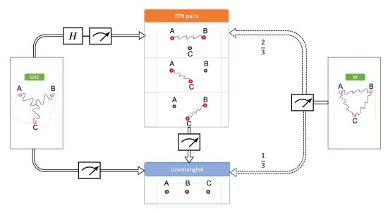
**Figure 5:** Distillation of EPR pairs from GHZ and W states. Continuous line arrows denote transitions with a deterministic outcome. Conversely, dotted line arrows denote transitions with probabilistic outcome.
