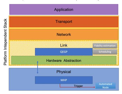
Figure 11: Schematic representation of the layered model proposed by Wehner et al., redrawn from [88].
