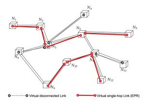
(b) Virtual Graph, representing the virtual connectivity within the network. In the example, although node  $N_6$  is physically connected to  $N_3$ , it does not belong to the virtual graph as it does not share an EPR pair. Hence, the virtual link between  $N_3$  and  $N_6$  is disconnected.
