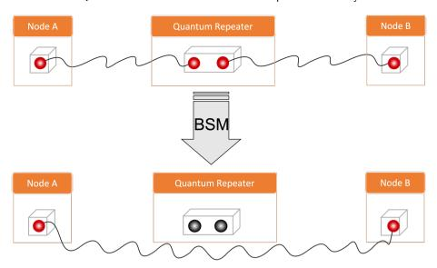
Figure 6: Pictorial representation of the entanglement swapping. By performing a BSM
