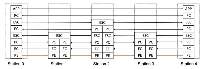
Figure 10: Example of layer interaction according to the Van Meter *et al.* protocol stack, redrawn from [82]. The physical entanglement (PE) layer and the entanglement control (EC) layer act recursively on single-hop links. Differently, the upper layers – i.e., the purification control (PC) layer and the entanglement swapping control (ESC) layer – act recursively on multi-hop links.
