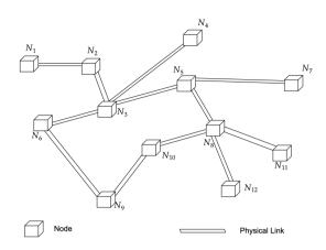
(a) Physical Graph, representing the physical connectivity within the network. In the example, Nodes  $N_3$  and  $N_6$  are connected by a physical communication link.
