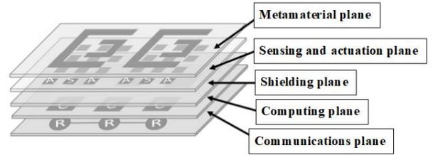
Fig. 12. Diagram of the general structure of an SDMs which denotes actuators-A, sensors-S, controllers-C and routers-R [83].
