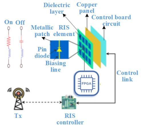
Fig. 8. Hardware model of RIS [61].
