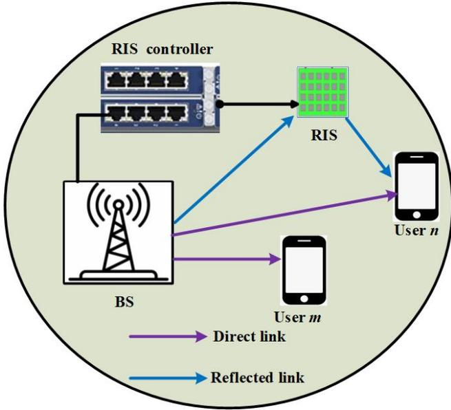
Fig. 32. Illustration of joint transmit and passive beamforming design.
