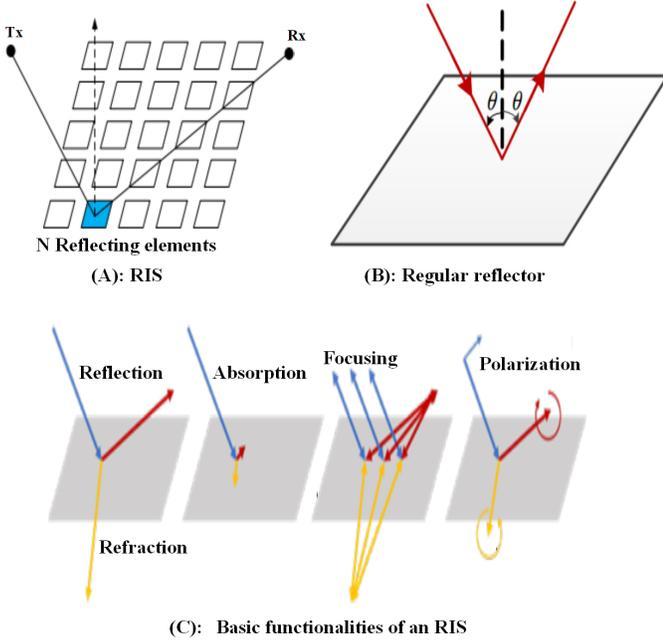
Fig. 6. The working principle of RIS.
