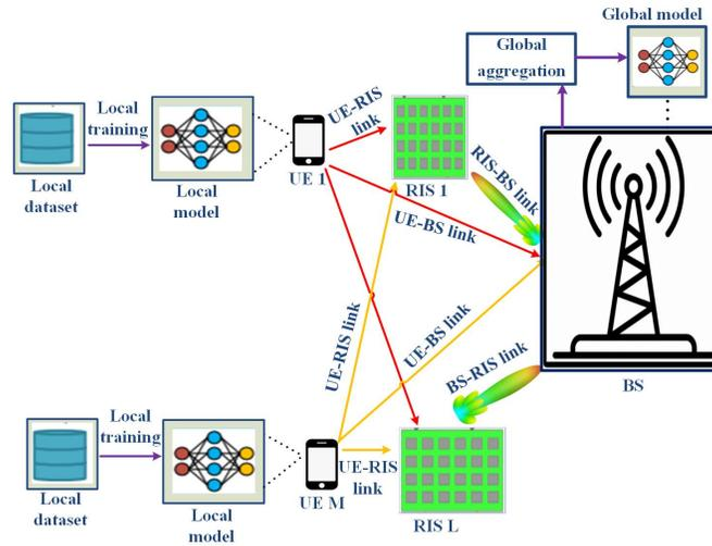
Fig. 19. A diagram of FL in multi-RIS assisted cellular networks [106].
