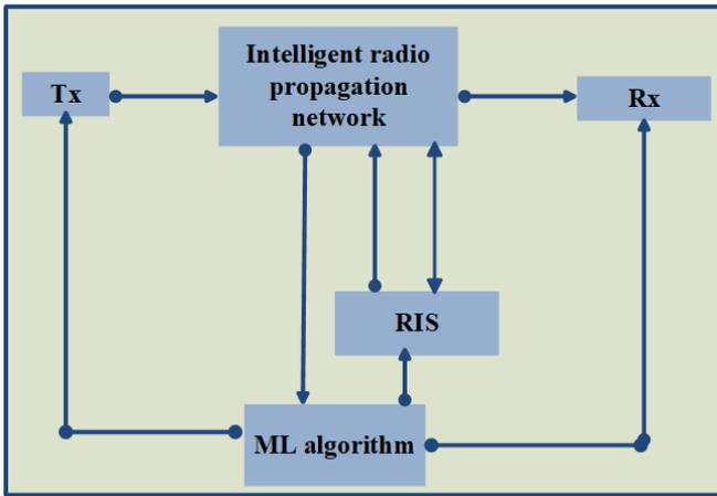
Fig. 4. Paradigm of configuring an intelligent radio propagation environment.
