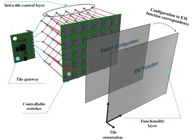
Fig. 13. Architecture of SDMs for IoT networks [25].
