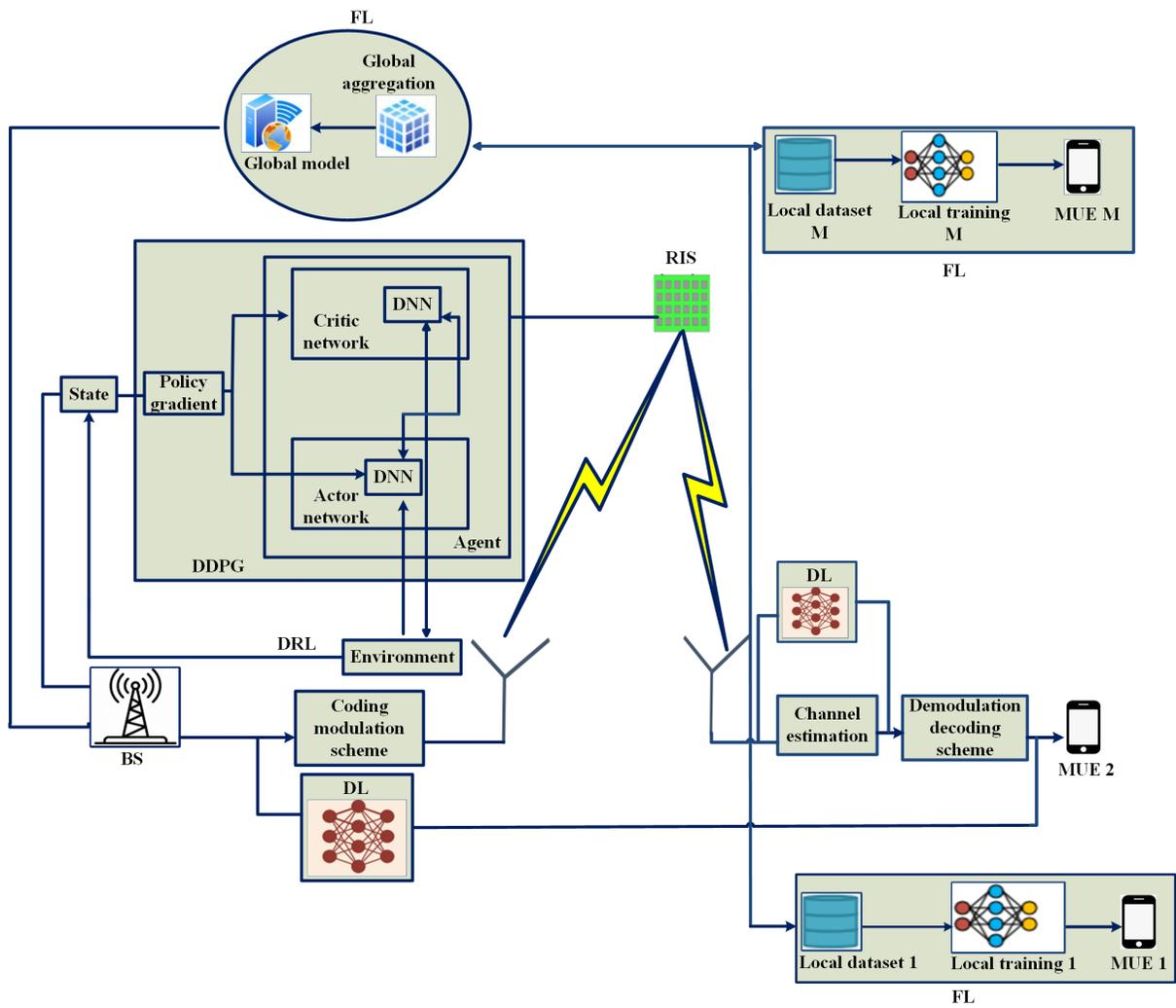
Fig. 23. Architecture of the ML embedded RIS-assisted M2M communications system.
