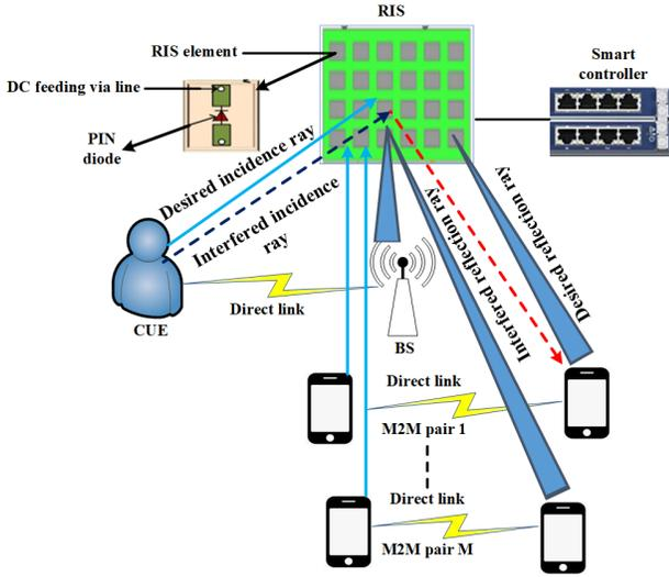
Fig. 21. RIS based M2M communications.
