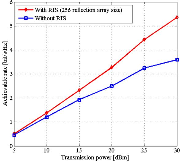
Fig. 10. Comparison of variation of achievable rate with transmission power.
