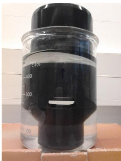
Fig. 9. The autonomous sensor immersed in a saline solution for lab tests.
