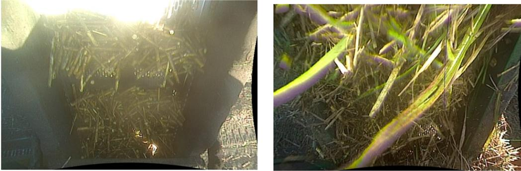
**Figure 19** Left: Sunlight washing out portion of the images. Right: Trash flying up and blocking the view of the camera.
