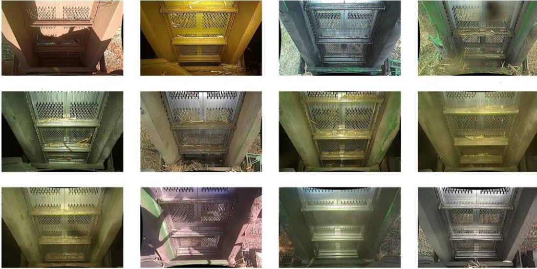
**Figure 6** Empty elevator images with various colors and under different lighting conditions.
