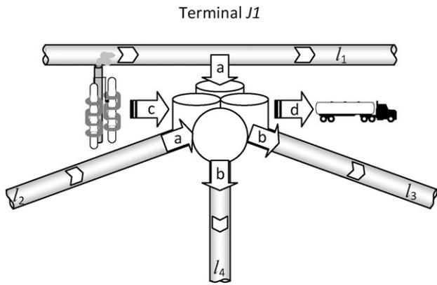
Fig. 3. Flow scenario for a generic terminal in the pipeline network.
