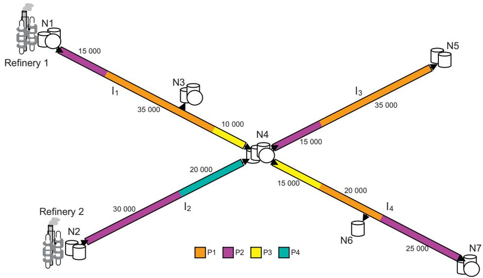
Fig. 6. Initial state of the multiproduct pipeline network of example 1.
