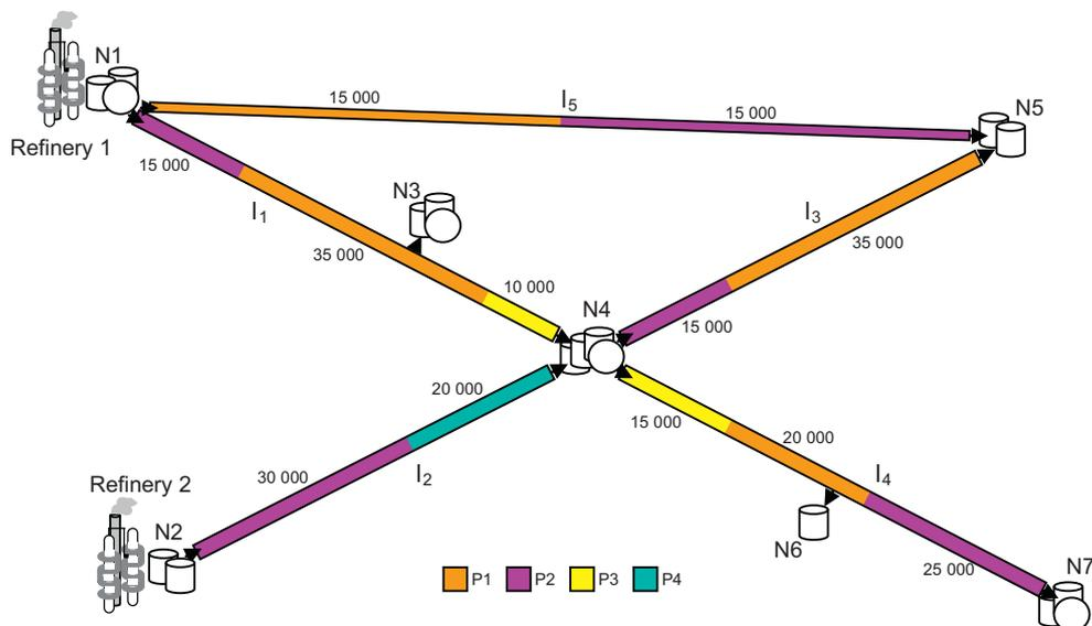
**Fig. 9.** Initial state of the multiproduct pipeline network of example 2.
