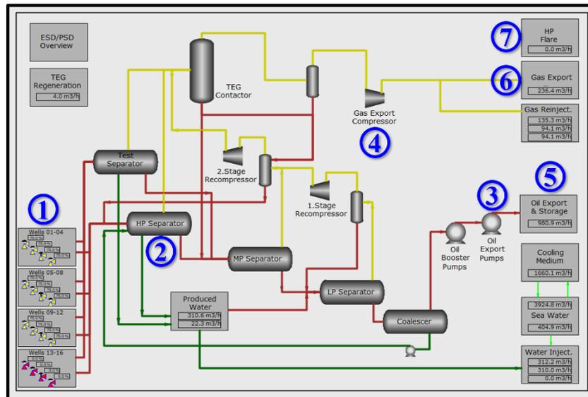
Figure 4. Overview of the generic oil and gas production process and monitored variables.
