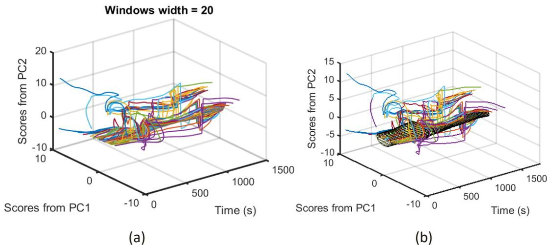
Figure 6. (a) SC2 – Scores from PC2 vs Scores from PC1 vs Time / (b) SC2 – Data-enclosing tunnel and training data.
