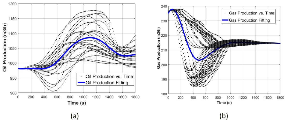
Figure 8. (a) SC1 – DEB1 – Curve fitting of the variable oil production / (b) SC2 – DEB1 – Curve fitting of the variable gas production.
