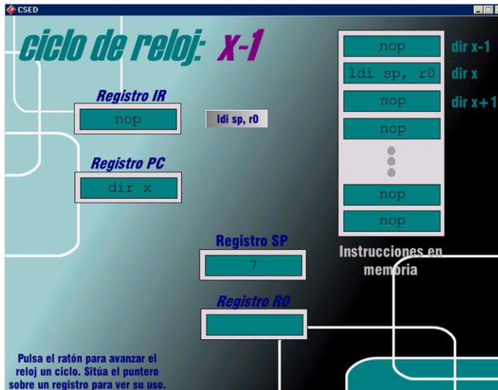
Fig. 8. Register addressing mode.
