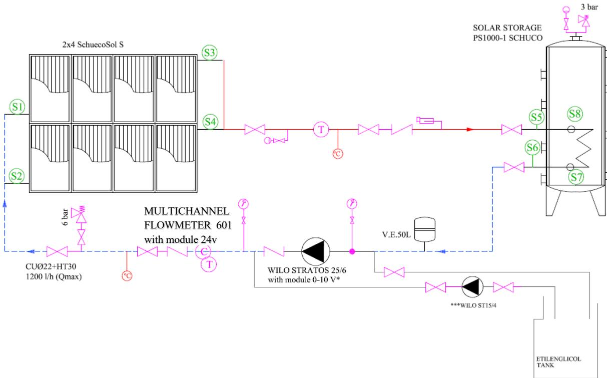
**Fig. 2.** Case Study under analysis: solar thermal system.
