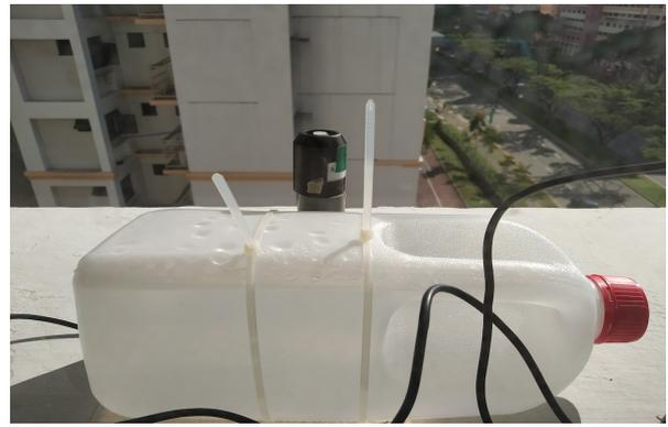
(b) PAR sensor placement on the window ledge.
