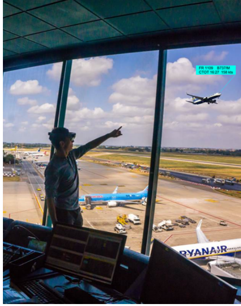
Fig. 1 An operator with the head-mounted display and the displayed information seen superimposed through the window (taking off flight identification and status)
