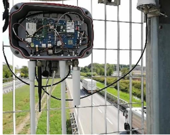
Figure 7: A Road Side Unit supporting C-Road Day 1 services installed along the Florence – Livorno freeway.
