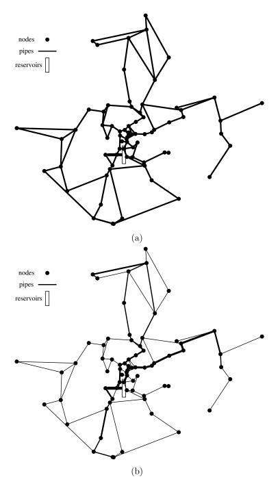
Figure 1: Example of a water distribution network. Demand nodes are represented as dots, reservoirs as rectangles and pipes as lines. The thicker lines represent larger diameter pipes. A network which is not optimized is exemplified in (a), whereas an optimized network is illustrated in (b).
