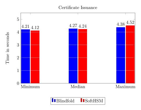
Figure 6: Time measurements of certificate issuance from Boulder integrated with Blindfold and SoftHSM
