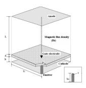
Fig. 3. Schematic diagram of the 1/4 simulation domain for a typical CNT-based triode-type field emitter within a periodic cell. Important geometrical parameters are: R=500nm, r=10nm, he=600nm, h=500nm, d=200nm, L=0.9mm and W=0.3mm.
