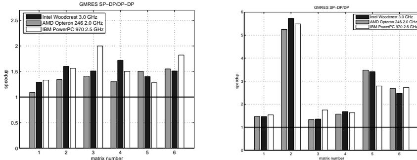
Figure 3: Mixed precision iterative refinement with FGMRES-GMRES<sub>SP</sub> from Algorithm 2 *vs* FGMRES-GMRES<sub>DP</sub> (*left*) and *vs* full double precision GMRES (*right*).
