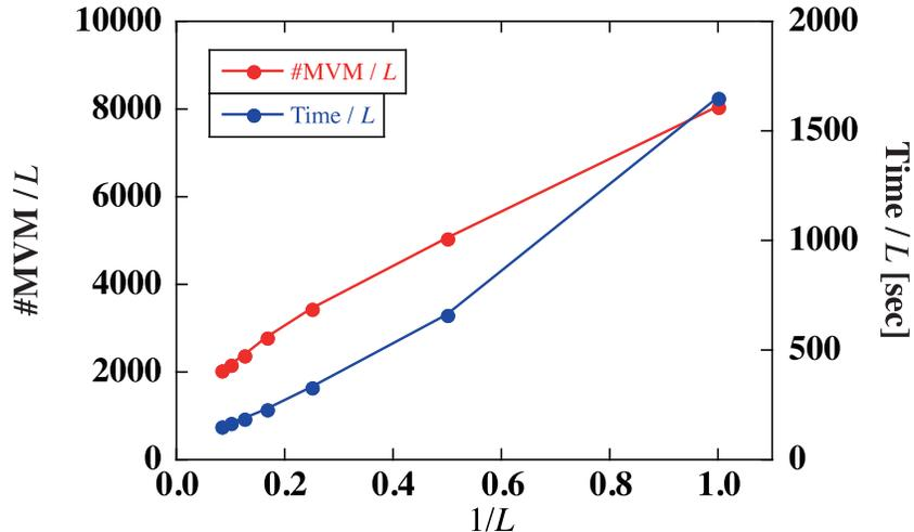
Figure 3:  $L$  dependence of  $\#MVM/L$  (red) and the execution time divided by  $L$  (blue) for the preconditioned block BiCGGR method with  $j = 12$ . All the results are averaged over 10 configuration samples.
