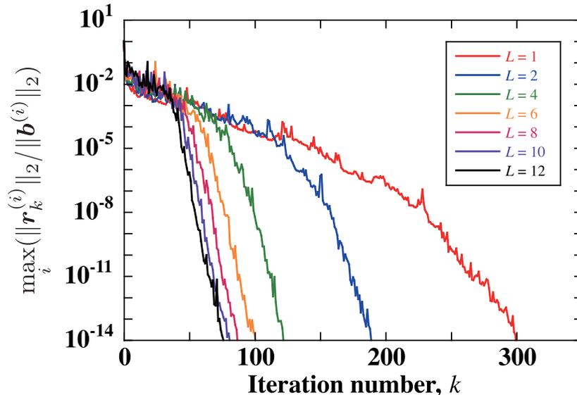
Figure 1:  $L$  dependence of the convergence behaviors for the  $j = 12$  case. All the measurements are performed on the same configuration.
