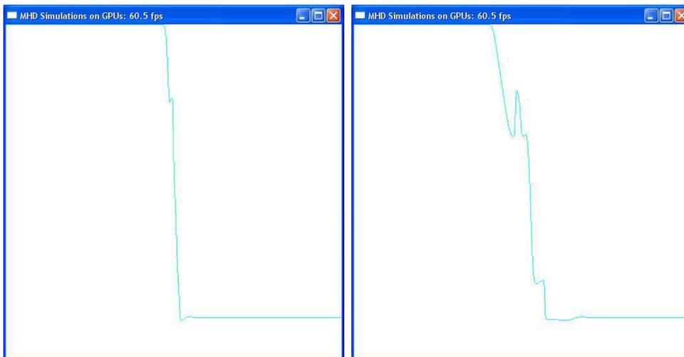
Fig. 25. 1D real-time visualizations of the density ( $\rho$ ) of Brio-Wu shock tube problem with 512 grid points using *GPU-MHD*.
