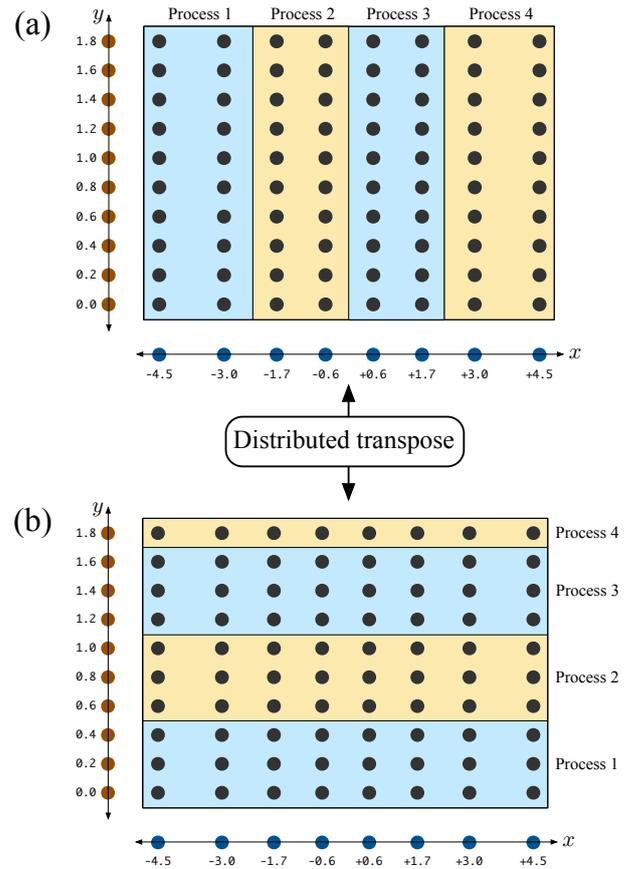
Figure 2: An example of problem parallelisation on a tensor product lattice. The problem is distributed across the (a)  $x$  or (b)  $y$  dimensions. These two problem decompositions are linked by a distributed transpose operation.
