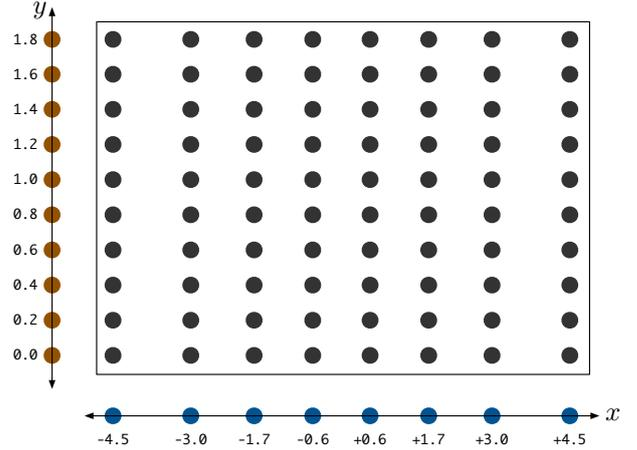
Figure 1: An example of a tensor product lattice. The specific unequal lattice spacing in the  $x$  direction is due to the fact that the basis functions in that dimension have been chosen to be Hermite-Gauss.
