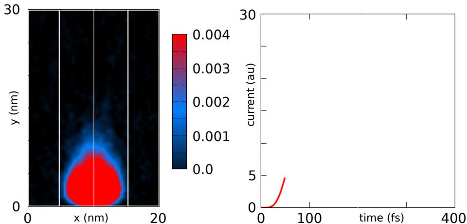
Figure 2: Density (in arbitrary units) after injection of 10 states (left). The potential walls and the middle of the wire are denoted by white lines. The current just begins to increase, which outlines the transient regime of the evolution (right).
