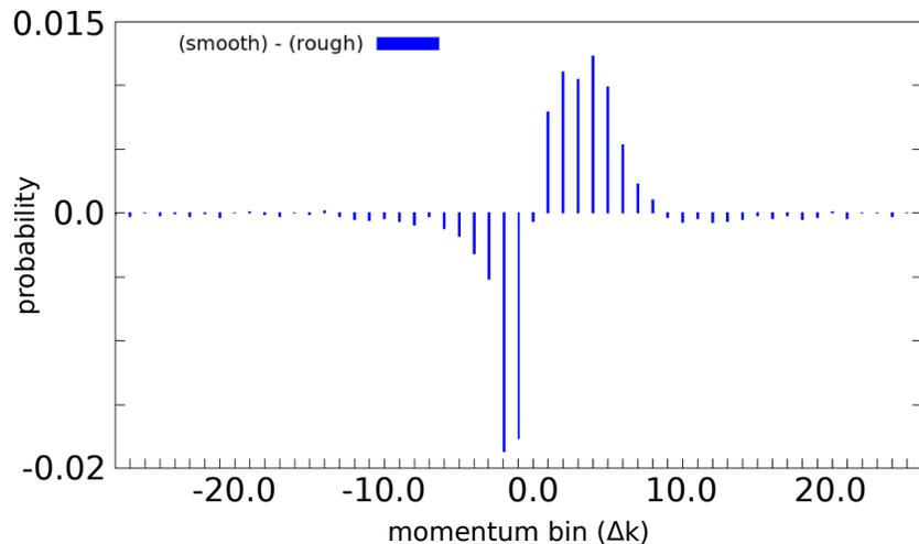
Figure 6: Difference of the ideal and rough marginal  $\mathbf{k}$  distributions in transport direction
