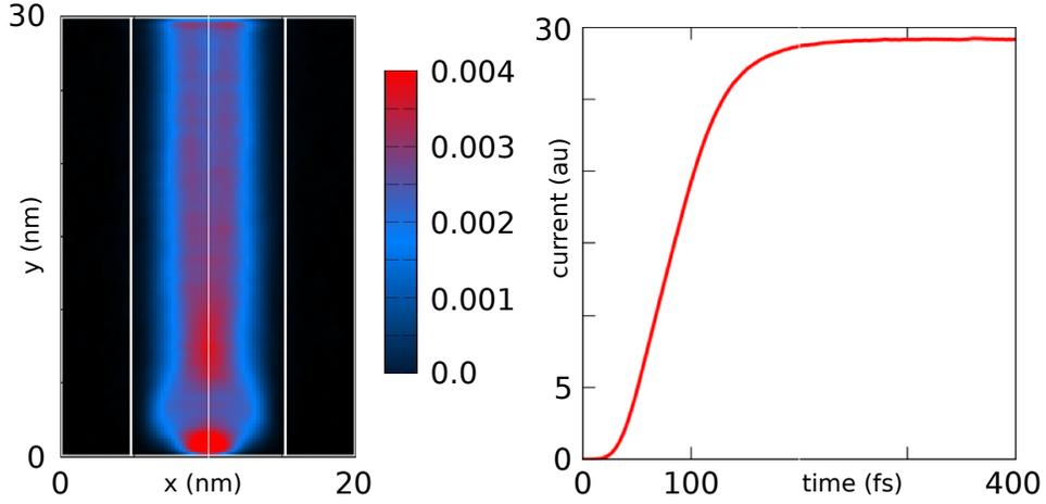
Figure 3: Density (in arbitrary unit) after 400fs evolution (left). The system enters into a stationary regime after 200fs, as seen from the current which remains constant during the next 200fs (right).
