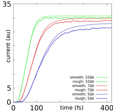
Figure 5: Current evolution in the ideal and rough wires for three different values of  $k_{0y}$ , corresponding to kinetic energies of 100meV, 50meV, and 25meV.
