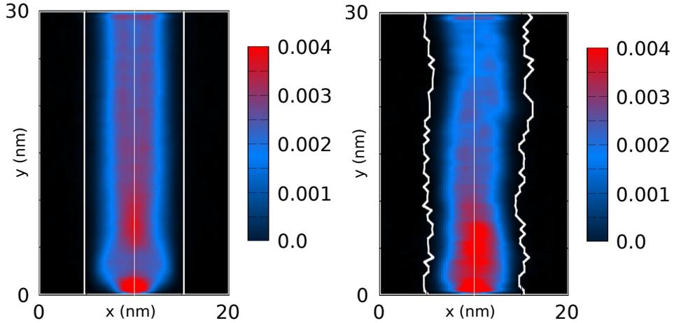
Figure 4: Density (in arbitrary unit) after 400fs evolution of the ideal (left) and the rough wire (right). Here  $k_{0y} = 5\Delta k$ , corresponding to an energy of 0.25meV.
