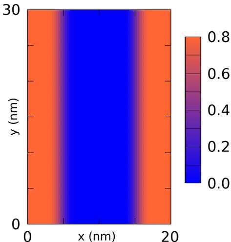
Figure 1: The wire is defined by two 0.8eV high and 5nm wide walls, which smoothly drop to zero within a few nanometers towards the middle of the channel.
