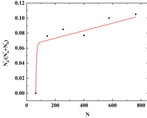
**Fig. 2.** The ratio  $N'_a / (N'_a + N'_b)$  of smaller particles to all particles in the red shaded, documented in Fig. 1, evolution versus  $N$ .  $N'_a$  and  $N'_b$  represent the number of small and large particles in the red shaded area, respectively.
