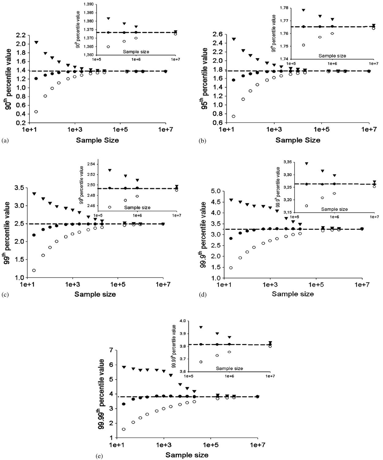
Fig. 13. Influence of the sample size on the 95% confidence interval and on the mean value of the some order statistics predicted by the GLD modeling of samples coming from  $GLD(0, 0.19, 0.14, 0.14)$  (their theoretical values are indicated by the horizontal dotted lines).
