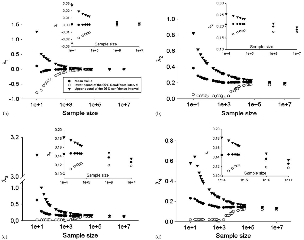
Fig. 15. The sample size versus the .025 and .975 quantiles of the sampling distribution and the mean value of the four GLD estimators calculated on samples coming from  $N(0, 1)$  and based on a bounded GLD.
