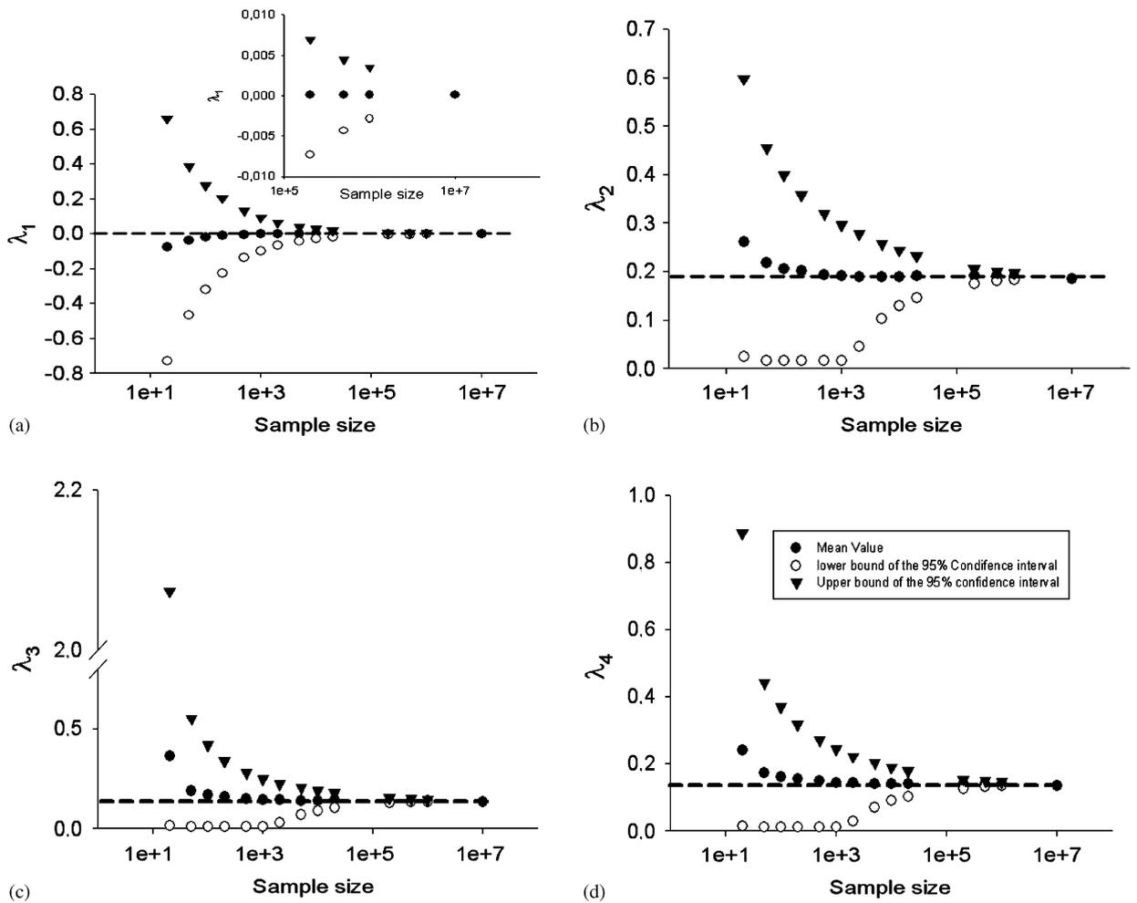
Fig. 7. Influence of the sample size on the 95% confidence interval and on the mean value of the estimates of the four GLD parameters for various sample sizes and when sampling coming from  $GLD(0, 0.19, 0.14, 0.14)$ . (Actual values are indicated by the horizontal dotted line.)
