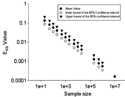
Fig. 10. Influence of the sample size on the 95% confidence interval and on the mean value of the  $E_{KS}$  distance calculated between the samples coming from  $GLD(0, 0.19, 0.14, 0.14)$  and their GLD modeling.
