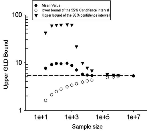
Fig. 8. Influence of the sample size on the 95% confidence interval and on the mean value of the upper bound of the GLD support calculated on samples coming from  $GLD(0, 0.19, 0.14, 0.14)$  and approached by a GLD (the theoretical value is indicated by the horizontal dotted line).
