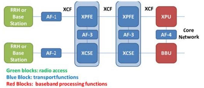
Figure 4: 5G-Crosshaul data plane architecture
