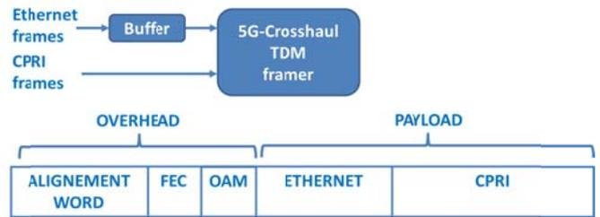
Figure 2: Simple TDM scheme for fronthaul and backhaul multiplexing
