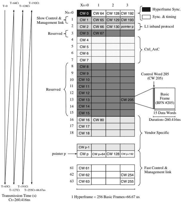
Figure 3: A simple TDM frame structure to multiplex fronthaul and backhaul traffic
