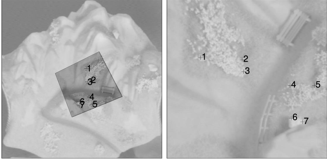
Figure 11: Example for the 3D scene “tunnel”. All of the 7 matches are correct. The estimated rotation angle is 77 degrees and the estimated resolution change is 3.2.
