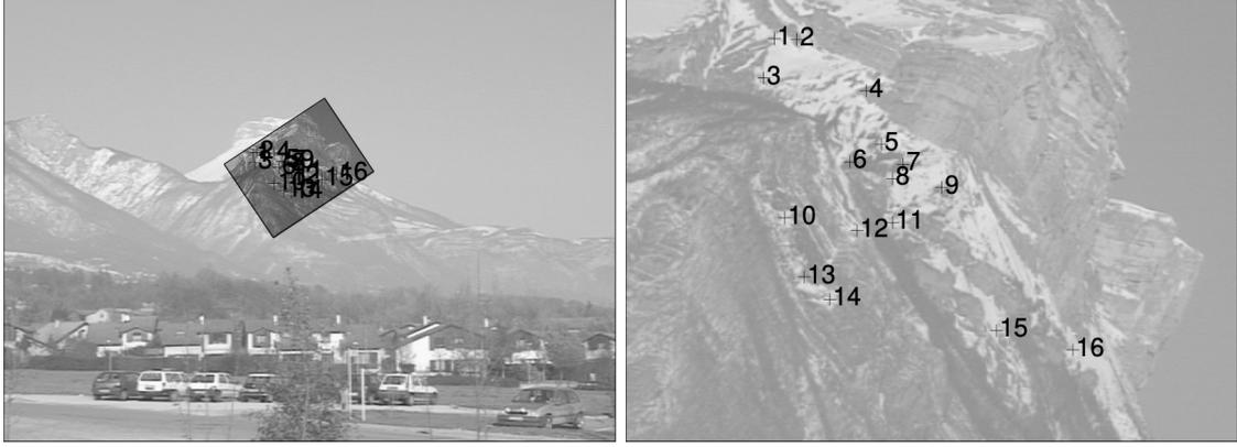
Figure 9: The final result obtained for the example in Figure 7. All of the 16 matches are correct. The high-resolution image is mapped onto the low-resolution one using the homography consistent with the 16 matches. The estimated rotation angle is 34 degrees and the estimated resolution change is 5.
