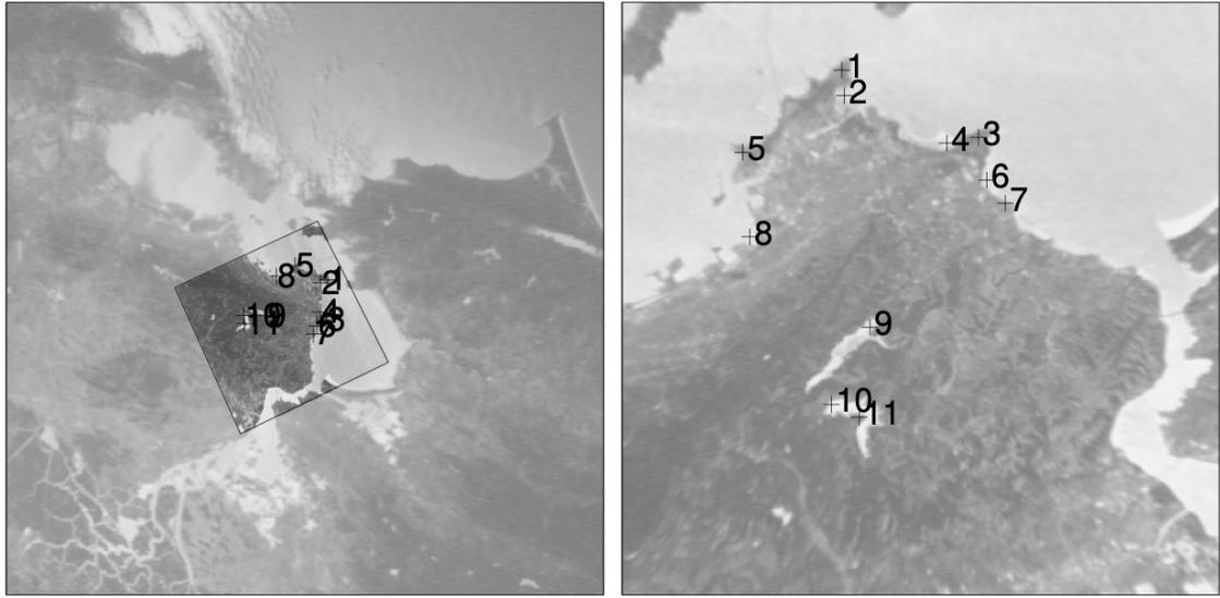
Figure 10: Example for a 2D scene. All of the 11 matches are correct. The estimated rotation angle is 65 degrees and the estimated resolution change is 3.7.
