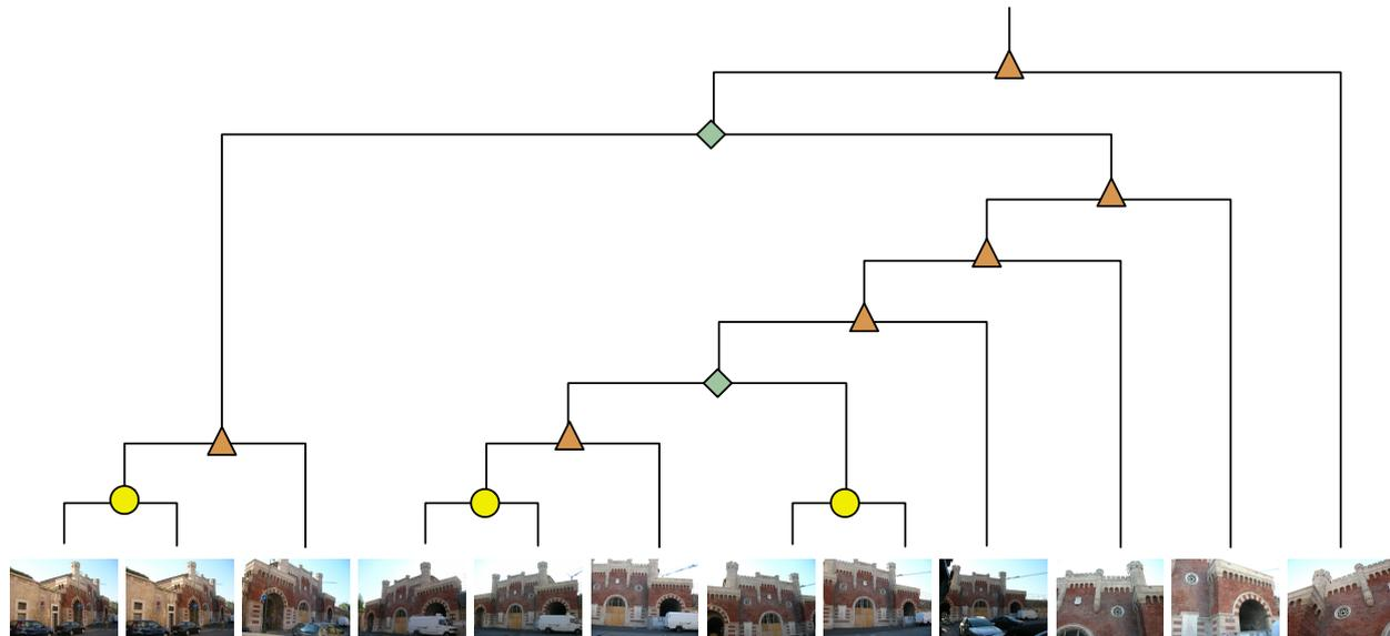
Figure 3: An example of a dendrogram for a 12 image set. The circle  $\bullet$  corresponds to the creation of a stereo-model, the triangle  $\blacktriangle$  corresponds to a resection-intersection, the diamond  $\blacklozenge$  corresponds to a fusion of two partial independent models.
